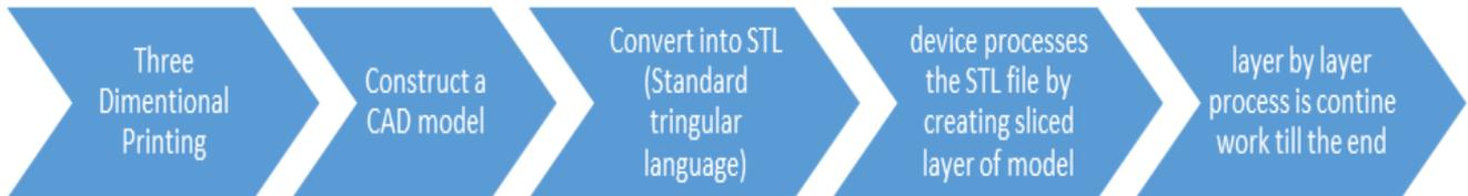
Fig. 2. 3D Printing Technique Basic Steps.
