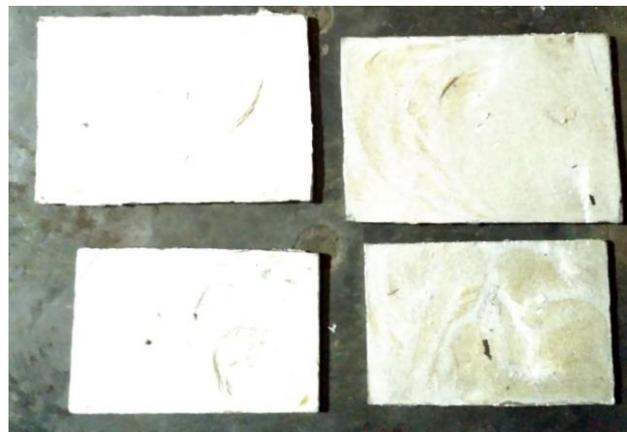
Fig. 5. Prepared 10%SiC Reinforced Al 6061 MMC.
