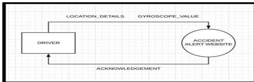
Fig. 1. Level 0 DFD (Data Flow Diagram)
