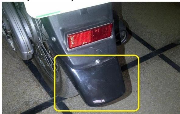
Fig.4.3 Mudguard with supplementary mudguard
