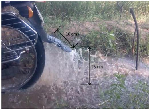
Fig.4.1 Experiments after additional mudguard
