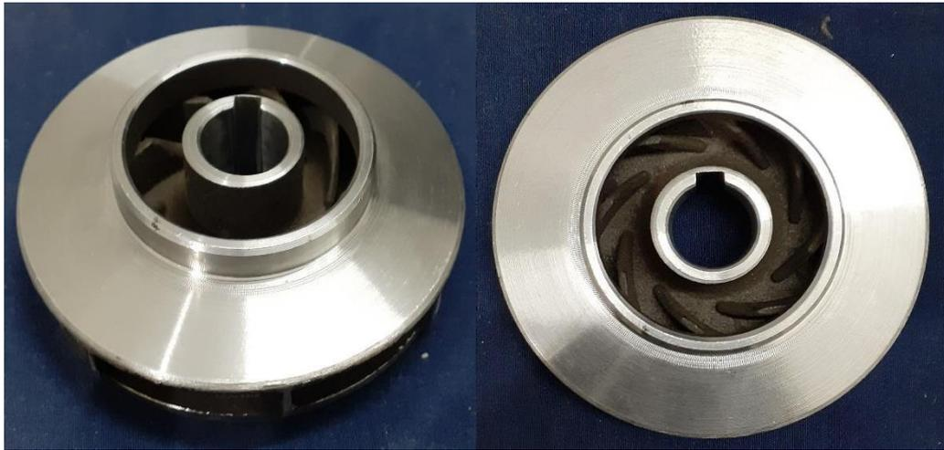
Fig. 3.0.1. Impeller manufacturing via sand casting method
